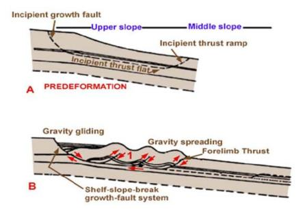
**Figure 1** - Stages of gravity tectonics/ gliding tectonics/gravity sliding, including a formation of detachment/decollement surfaces and formation of thin-skinned fold and thrust belts by gravity sliding. (<u>http://oilandgastraining.net</u>).
