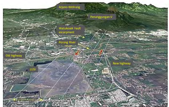
Figure 18. Satellite image oriented SW direction. The vast grey area is occupied by LUSI mud surrounded by embankment. To the SW, geomorphic of river become the evidence of sinistral-strike slip fault as denoted by abrupt changes of the Porong River, the prominent escarpment of Watukosek fault, the neighbouring Penanggungan volcano (that lies approximately ~10 km away) and the Arjuno-Welirang volcano complex. Four white dashed lines notifies the intersected area of sinistral strike-slip fault system of Watukosek. Note that several natural features as mentioned above are controlled by the fault system (Miller and Mazzini, 2018).
