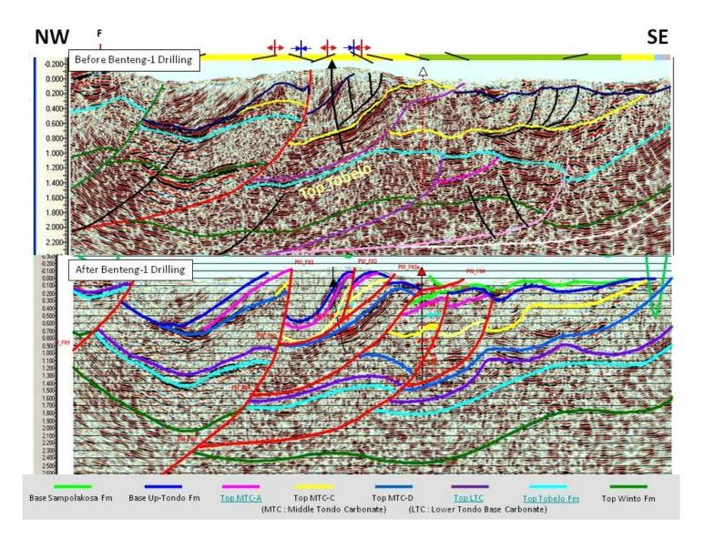
Figure 8 - Seismic sections interpreted before and after drilling Benteng-1 well (Japex, 2012). The deformation is much more complicated than prognosed, making Tobelo objective could not be penetrated due to much deeper than prognosed. Seismic data was acquired in 2008, poor quality due to complicated deformation.
