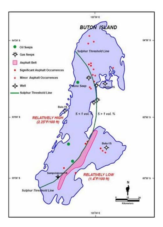
Figure 4a - Asphalt belt of Buton occurring at the southern part of the island.
