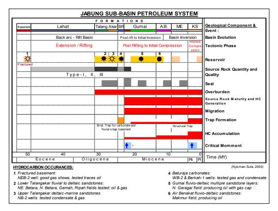
FIGURE 11 : Petroleum system of the area showing base Gumai source rock potential in relation to other geologic element / events.
