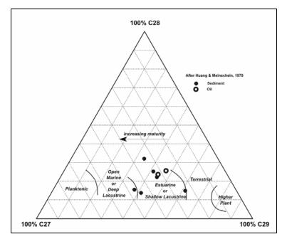
**FIGURE 7 :** Sterane distributions display concentration of C<sub>27</sub>-C<sub>29</sub> forms consistent with mixed marine/terrestrial source kerogen
