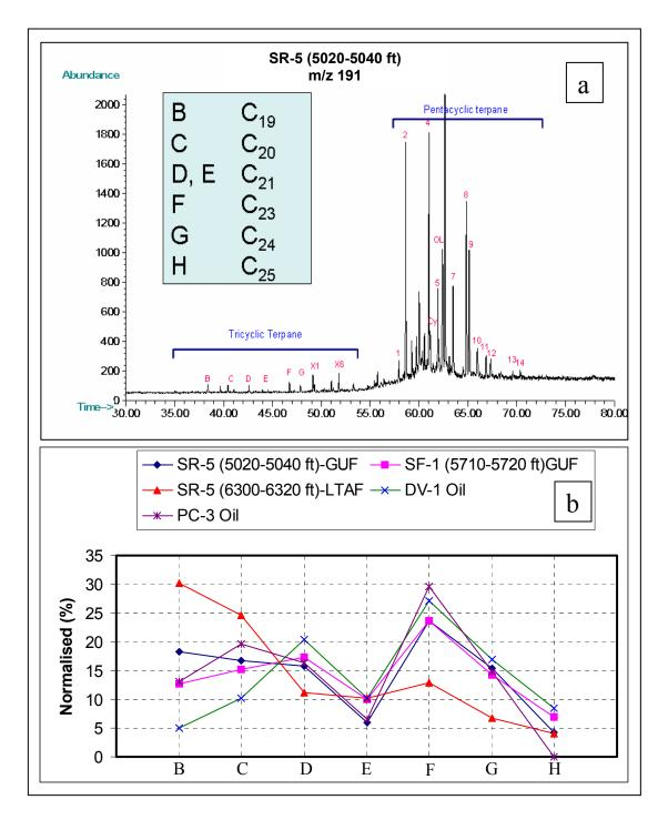
**FIGURE 9 :** (a) Saturate and aromatic carbon isotope-13 shows a mixed terrestrial and algal material, dominated with algal, (b) Distribution of tricyclic terpanes show a correlation between oil and sediment from Gumai Formation and compare to Lower Talang Akar sediment
