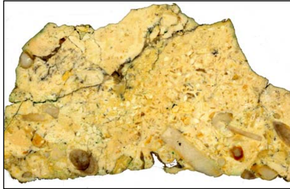
Figure 5. Polished slab of sampel from Sodong shows very coarse bioclastic grained packstone consisting of abundant large foraminifera, coral fragments, red algae, and echinoid spines.
